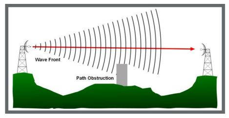
Figure 1: Example of diffraction due to Fresnel obstruction
