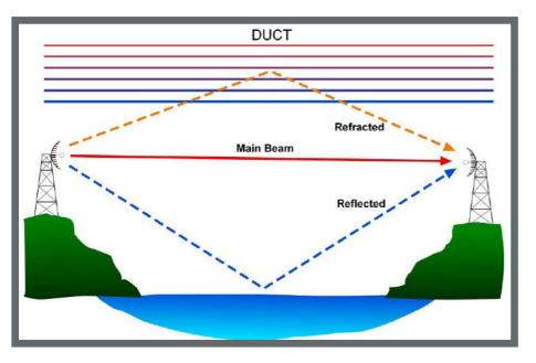
Figure 4: Reflected and refracted multipath
